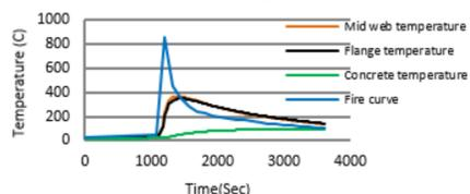
Significant residual strength reduction of concrete or the steel cannot happen in the structure. Bottom surface temperature up to 250°C could result in localized cracks and dehydration of the cementitious paste with complete loss of free moisture which could lead to spalling of concrete.
