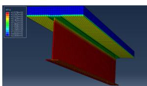
Fig. 4. 3-D Abaqus Model of the structural element used for the heat transfer analysis
