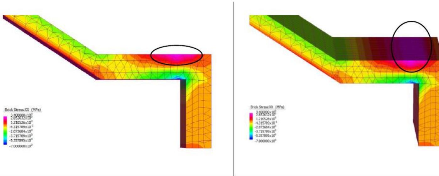
Figure 5.2: Critical Tensile Stress Region – Horizontal Leg
