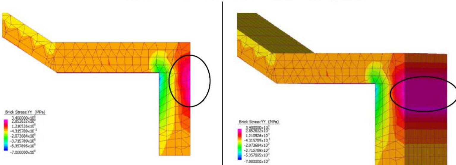
Figure 5.3: Critical Tensile Stress Region – Vertical Leg
