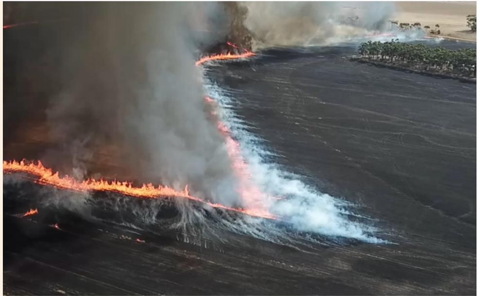
▲ **Above:** THIS RESEARCH USED FIELD-SCALE EXPERIMENTS AND DRONES TO TRACK THE WAY THAT MERGING FIRE FRONTS BEHAVE. PHOTO: BRETT CIRULIS.
