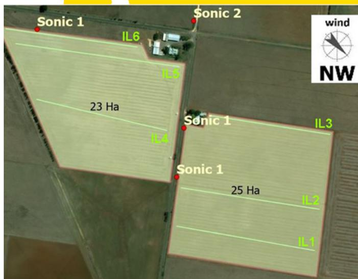
▲ **Figure 1:** LOCATION OF EXPERIMENTAL PLOTS. GREEN LINES AND RED DOTS REPRESENT IGNITION LINES AND SONIC SENSORS, RESPECTIVELY.
