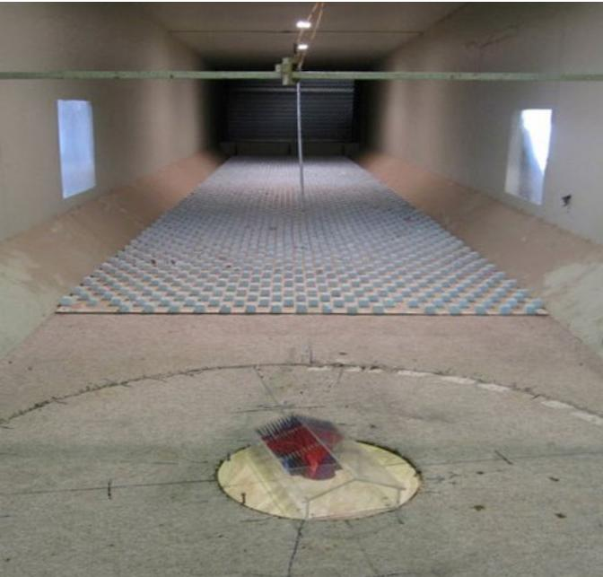
Tests in Wind Tunnel at the Cyclone Testing Station, James Cook University. On representative houses at a length scale ( $L_r$ ) of 1/50
