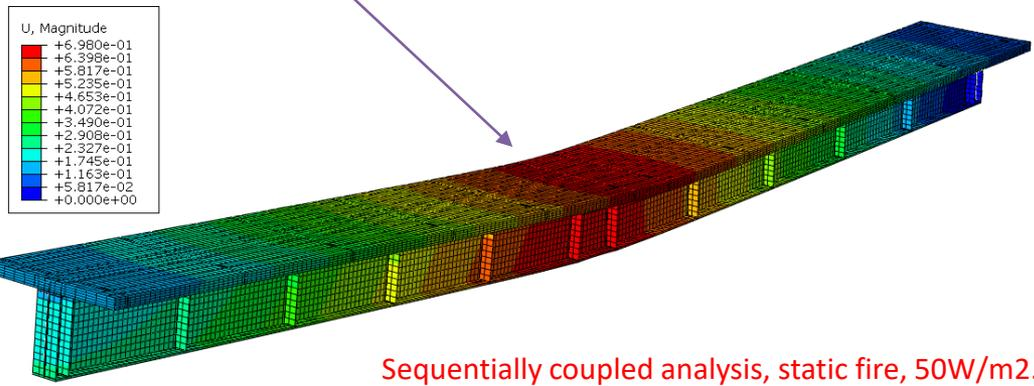
Sequentially coupled analysis, static fire, 50W/m<sup>2</sup>.C conv.ht.coef.
