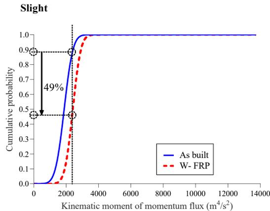
The reduction in probability of failure using FRP wraps is more pronounced at the extensive damage state (i.e. drifts at peak in capacity curves)
