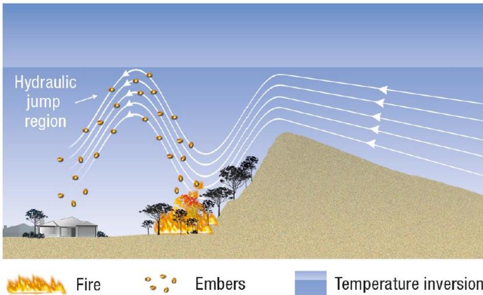
Figure 6. Schematic depicting transport of embers by downslope winds where the embers are lofted by the hydraulic jump then deposited on properties.
