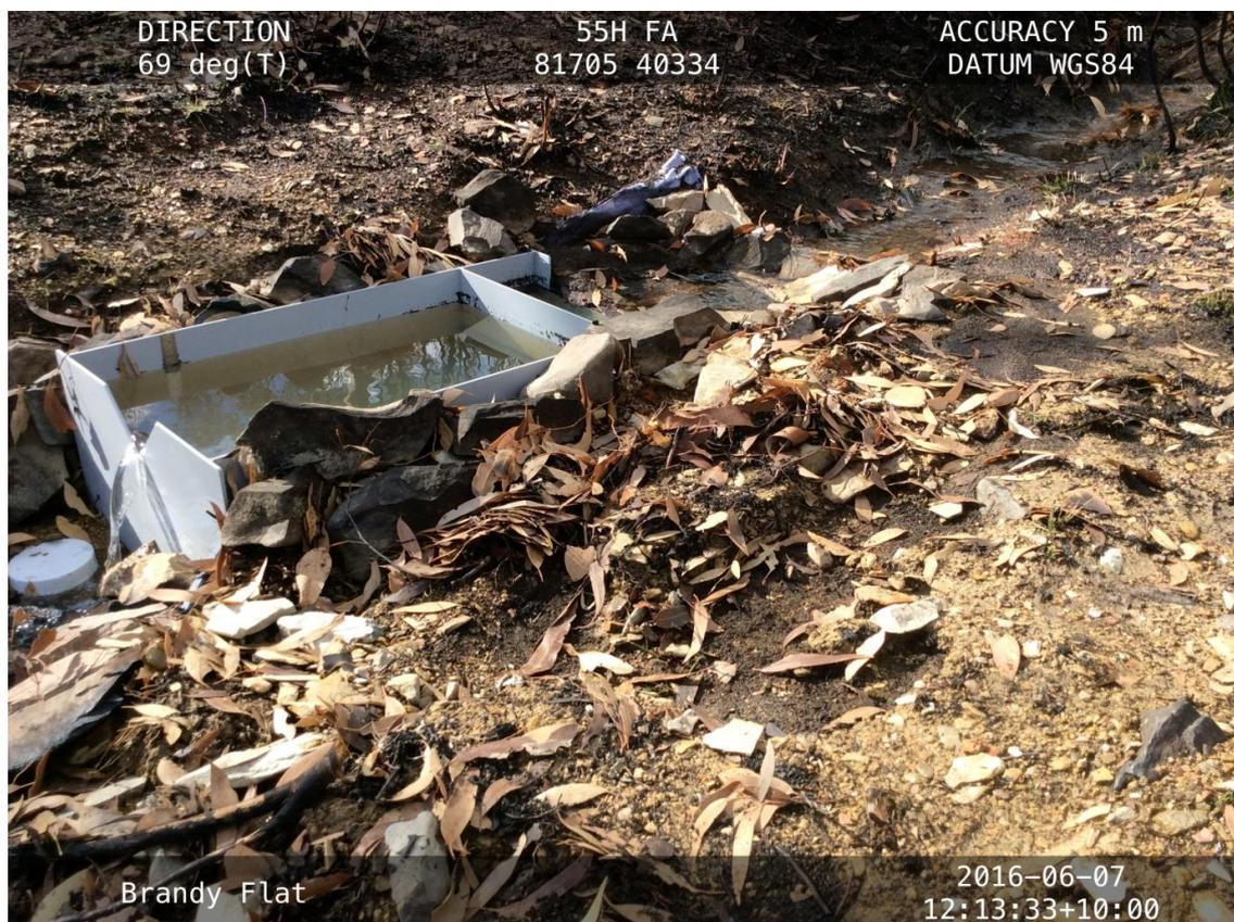
FIGURE 3 - A SEDIMENT TRAP AND A V-NOTCH WEIR INSTALLED IN A BURNED GULLY
