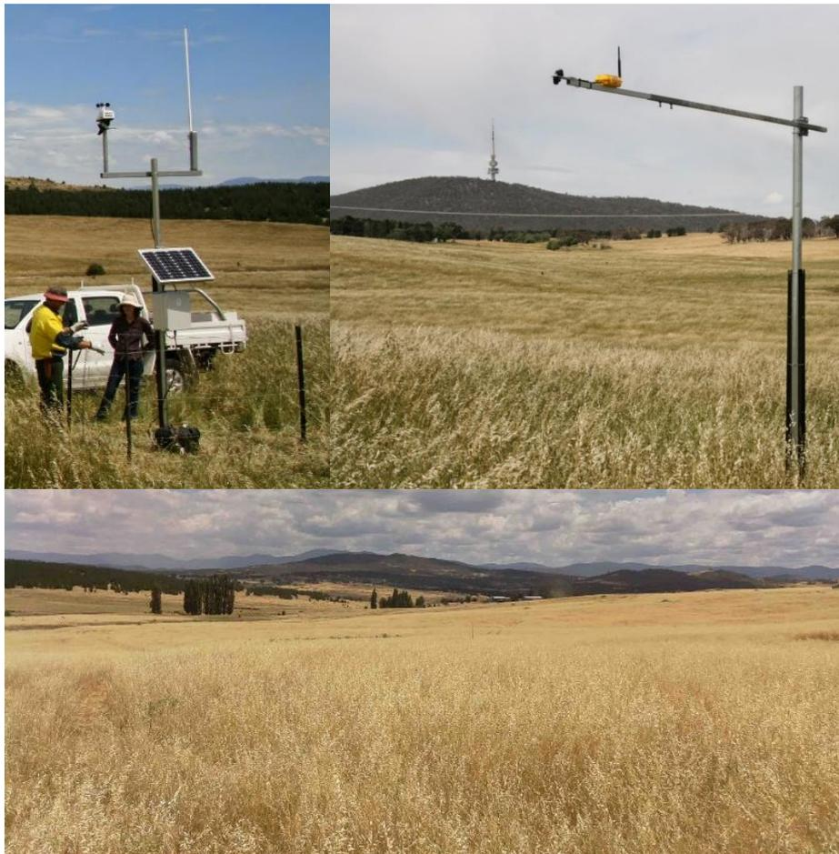
FIGURE 11. IN-SITU SENSORS FOR MONITORING GRASS CURING AND FUEL MOISTURE CONTENT. (TOP LEFT) METEOROLOGICAL STATION; (TOP RIGHT) ONE OF THE 5 SENSOR LOCATED ON THE SITE AND (BOTTOM) VIEW FROM THE RASBERRY PI CAMARA.
