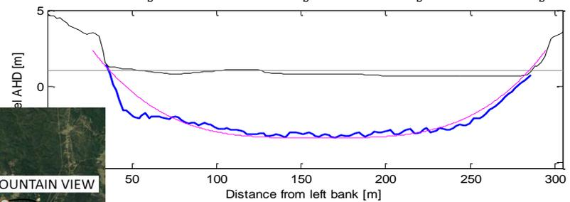
Cross section N. 36 - Depth<sub>b</sub> = -11.9356m ; meanDEPTH<sub>b</sub> = 7.2196m; WIDTH<sub>b</sub> = 151.2115m; AREA<sub>b</sub> = 842.325m<sup>2</sup>
