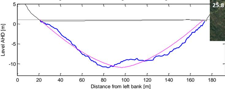
Cross section N. 48 - Depth<sub>b</sub> = -11.6256m ; meanDEPTH<sub>b</sub> = 6.664m; WIDTH<sub>b</sub> = 198.5907m; AREA<sub>b</sub> = 1323.3992m<sup>2</sup>
