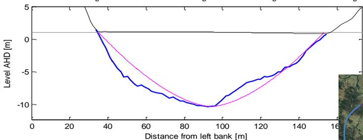
Cross section N. 49 - Depth<sub>b</sub> = -4.4042m ; meanDEPTH<sub>b</sub> = 3.2492m; WIDTH<sub>b</sub> = 247.6307m; AREA<sub>b</sub> = 804.5948m<sup>2</sup>
