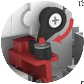
The servo mechanism trips and releases the paddle, simulating flow and sending the status to the monitoring system, all while the system remains closed. Potter's proprietary algorithm ensures water is present in the system.
