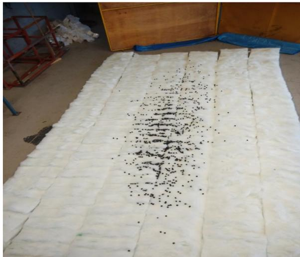
Figure 7. Results from a very preliminary experiments on the distribution of embers emanating from a prototype firebrand generator.
