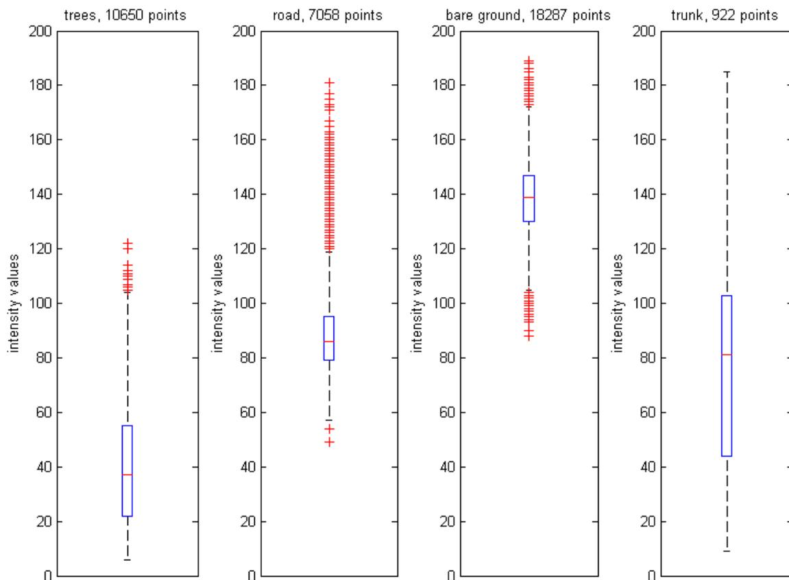
Figure 12. Boxplots showing the distribution of the intensity values over four classes of materials: trees, road, bare ground and trunk. A difference in intensity values is apparent between the different materials (Source [1])
