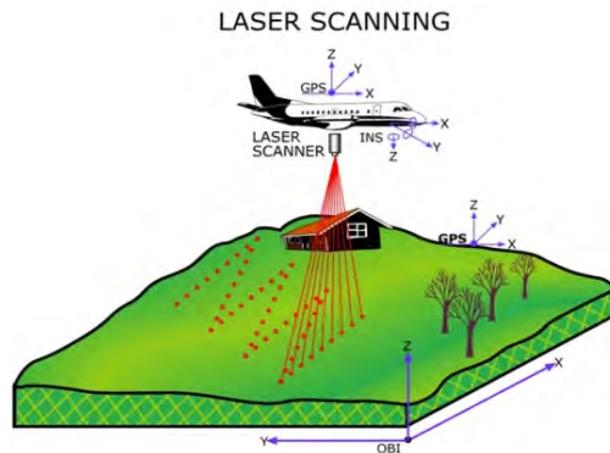
Figure 1. To determine the precise location (that is, georeference) of LiDAR points, use is made of global positioning systems (GPS) to derive the position of the aircraft, a so-called inertial navigator that determine the pointing direction of the sensor, and the LiDAR range to extrapolate the coordinates of a target point on the ground (source: ASPRS).
