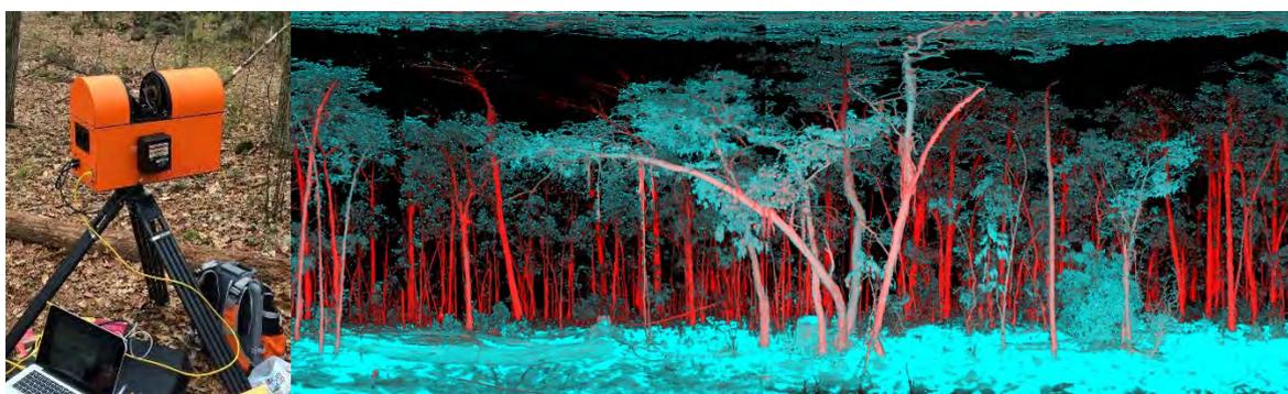
Figure 13. New DWEL laser scanner (left) and a normalized normalised difference index (NDI) image of the woodlands of Mulligans Flat Natural reserve produced by the DWEL (right). NDI was computed using the laser reflectance at 1064nm and 1556nm. The NDI image easily define the trunks and the leaves. Very “green” vegetation should appear blue, Red sections of the image relate to non-green vegetation components. Courtesy of Michael Schaefer.
