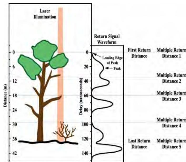
Figure 3. Full-wave LiDAR vs discrete multiple-return LiDAR. In full-waveform LiDAR, the entire return pulse is digitized and recorded. In a discrete multiple-return LiDAR, only the peaks are recorded. Source: ASPRS.
