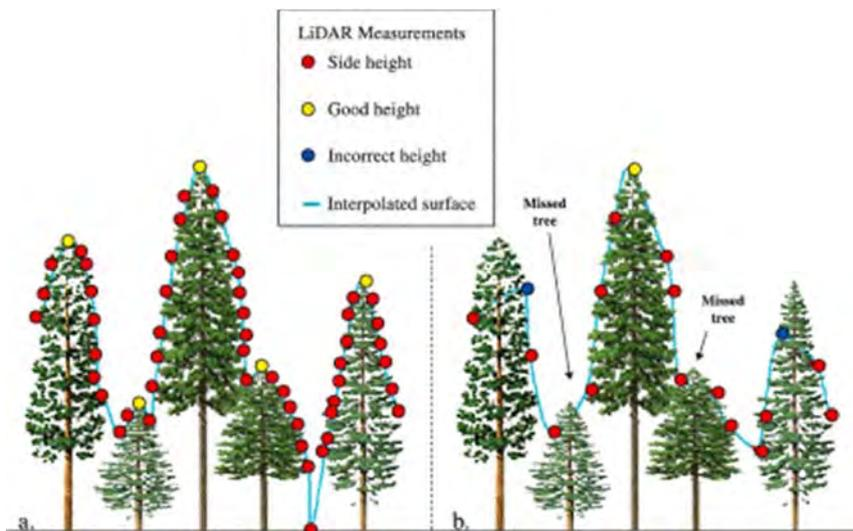
Figure 5. (a) Accurate estimate of tree height dispersion due to a high point density. (b) Less accurate estimate of tree height dispersion due to low point density (source [10]). Higher point density yields better accuracy in detecting the dispersion of tree heights.
