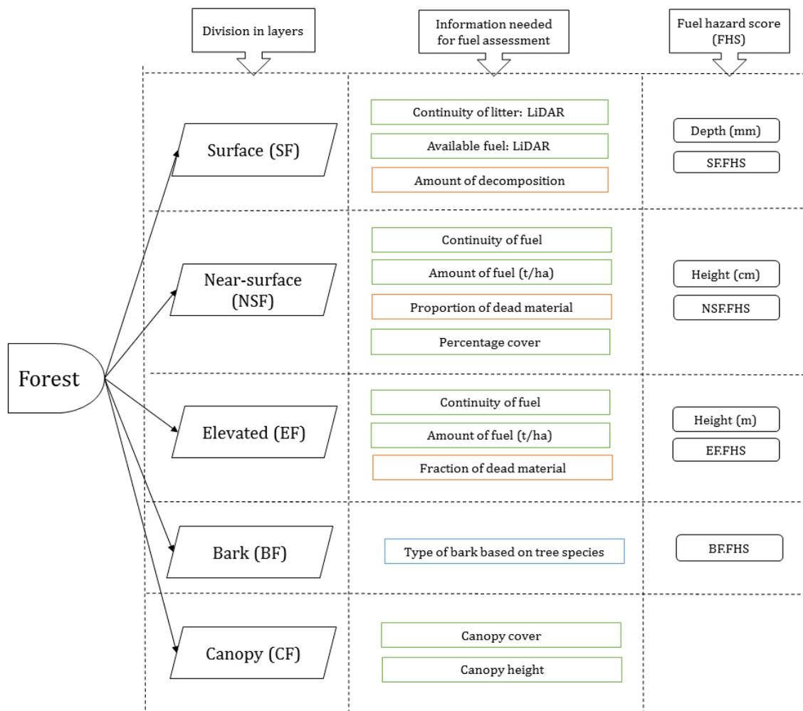
Figure 18: Theoretical framework on how to derive the variables needed for a fuel assessment from LiDAR (green) and hyperspectral (orange) data. Structural parameters on the different vegetation layers can be derived from airborne and terrestrial LiDAR data. Complementary hyperspectral data can be used to derive fuel moisture, amount of decomposition, proportion of dead material and even type of bark through species classification. Source, modified from [1].
