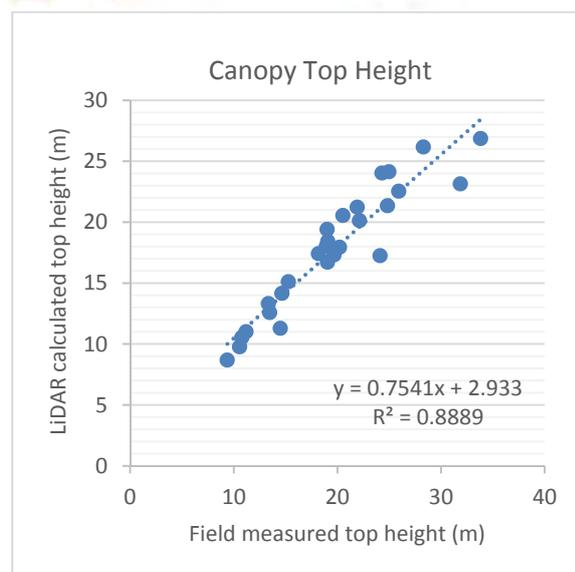
Figure 6: Canopy height map derived from discrete LiDAR ( $5 \text{ pt m}^{-2}$ ) for Mulligans Flat Nature Reserve, ACT (a). Correlation between field and discrete LiDAR derived tree height for 28 trees at Mulligan's Flat Nature reserve (b). This LiDAR data was acquired on December 2013. Source [1]
