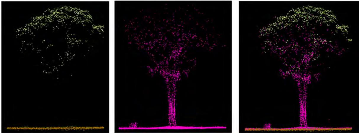
Figure 16. Airborne and ground-based LiDAR dataset complement each other very well since airborne LiDAR captures the canopy whereas ground-based LiDAR accurately measures the ground and elevated fuels. Source, [16] <http://www.bnhcrc.com.au/resources/poster/1233>.
