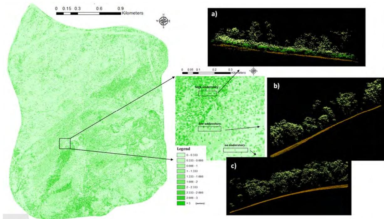
Figure 10. Discrete LiDAR-derived understorey height for the Black Mountain Reserve. Transect “a” shows that when the values are higher the understorey is higher. When the values are low the understorey is either absent (transect “c”) or almost absent (transect “b”) Source [1]
