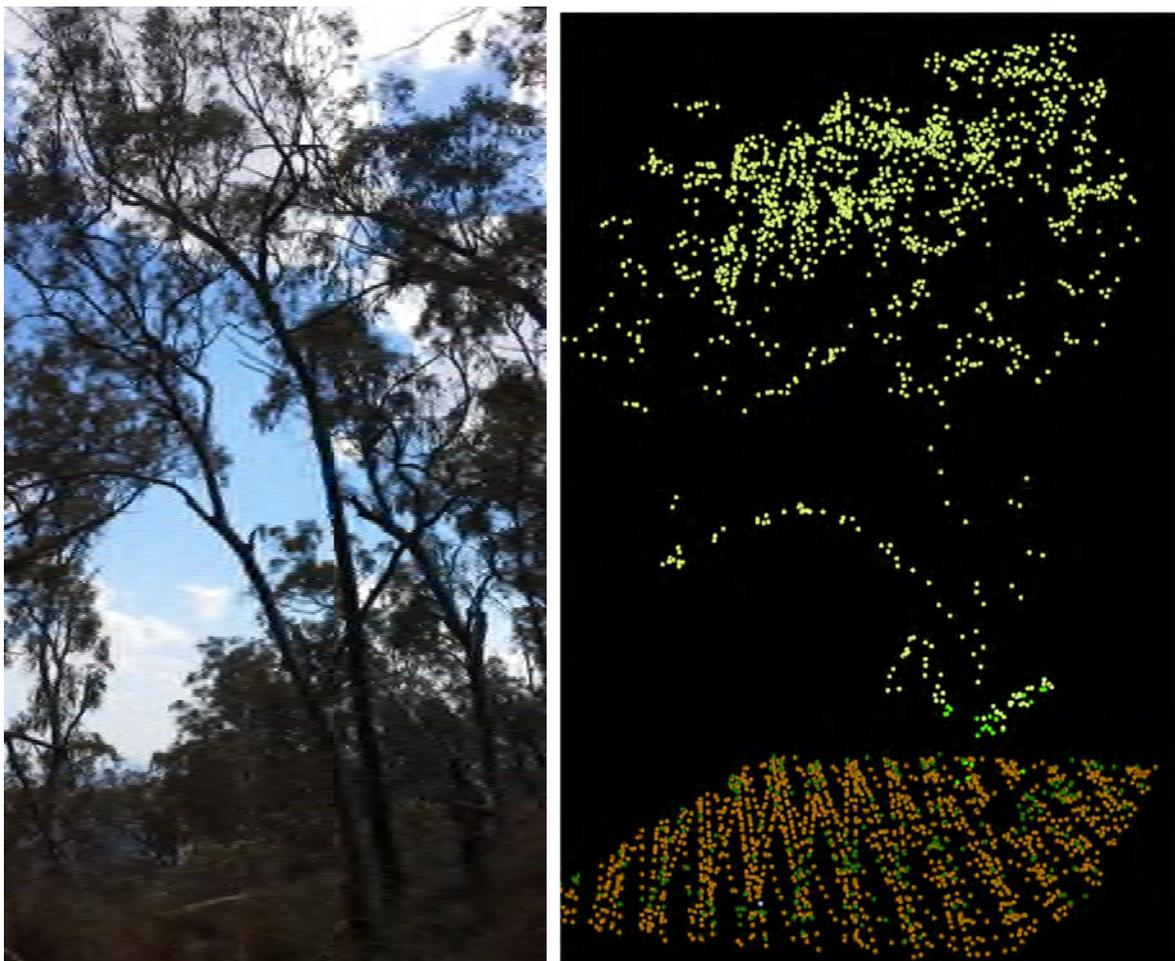
*Figure 9. The photo on the left shows a relatively open stand with ladder fuels and the photo on the right the way multiple discrete return LiDAR represents this stand.*
