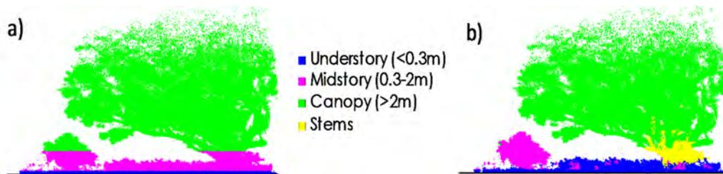
Figure 15. Fuel classification with Zebedee a) Based on the presence of points classified within a specific height layer b) using an algorithm that re-classifies the previous output based on forest fuels rules. The later better distinguishes between forest fuel layers with some minor noise. Source, [16] <http://www.bnhcrc.com.au/resources/poster/1233>.
