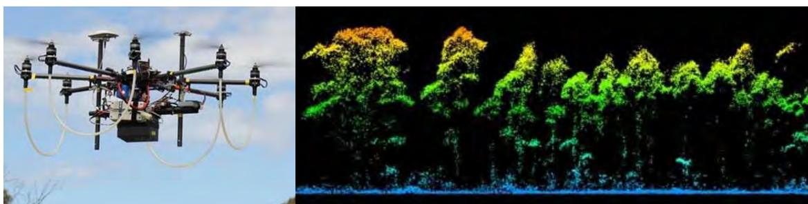
Figure 17. The multi-rotor Oktocopter UAV platform carrying the laser scanner (left), An example point cloud at an average point density of 40 points per square meter (right). Source [28].
