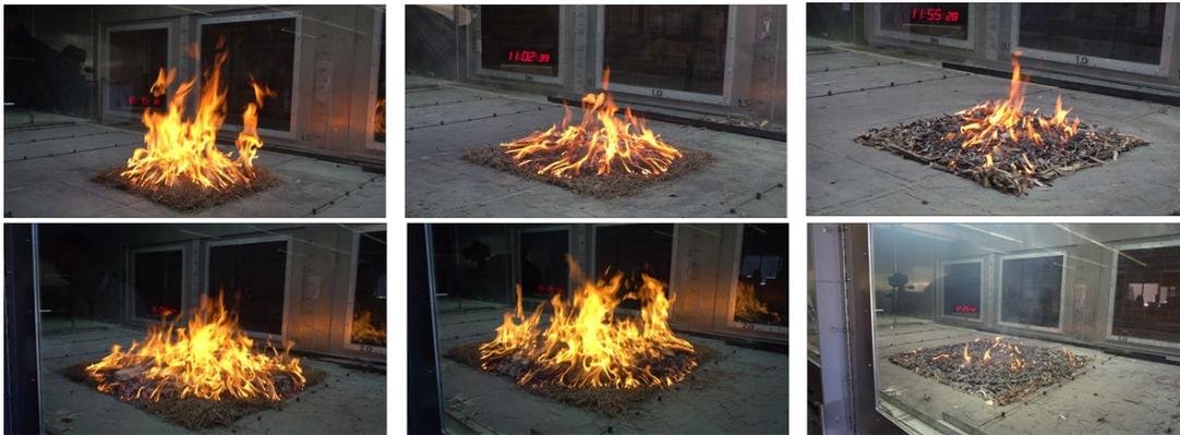
**FIGURE 16:** COMPARISON OF RELATIVE FLAME HEIGHTS ASSOCIATED WITH THE THIRD ROW OF IMAGES FROM FIGURE 14 (TOP ROW, 500 MM DIAMETER) AND FIGURE 15 (BOTTOM ROW, 1000 MM DIAMETER) FOR UNCOMPACTED PINE NEEDLES (LEFT COLUMN), COMPACTED PINE NEEDLES (CENTRE COLUMN) AND EUCALYPT LITTER (RIGHT COLUMN).
