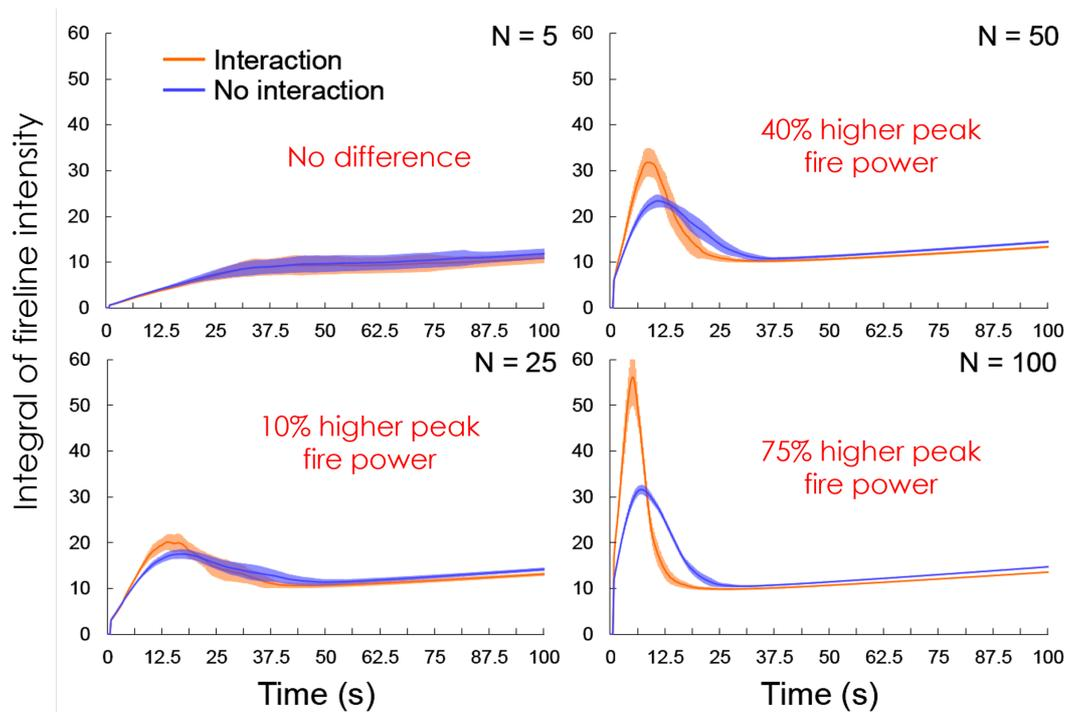
**FIGURE 10:** POWER PROFILE (INTEGRAL OF NON-DIMENSIONALISED FIRELINE INTENSITY) FOR RANDOMLY DISTRIBUTED COALESCING SPOT FIRES AS A FUNCTION OF DIFFERENT NUMBER OF SPOTS FIRES. THE LINES SHOW THE MEAN VALUE OVER TEN ENSEMBLE SIMULATIONS AND THE CONFIDENCE BAND SHOWS ONE STANDARD DEVIATION. FIGURE ADAPTED FROM HILTON ET AL. (2017).
