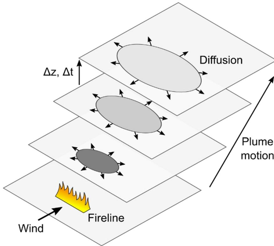
**FIGURE 23:** SCHEMATIC ILLUSTRATION OF PLUME DIFFUSION MODEL. THE HORIZONTAL TRANSECTS SHOW THE PERIMETER OF THE PLUME AT VARIOUS HEIGHTS AS IT DIFFUSES INTO THE SURROUNDING ATMOSPHERE
