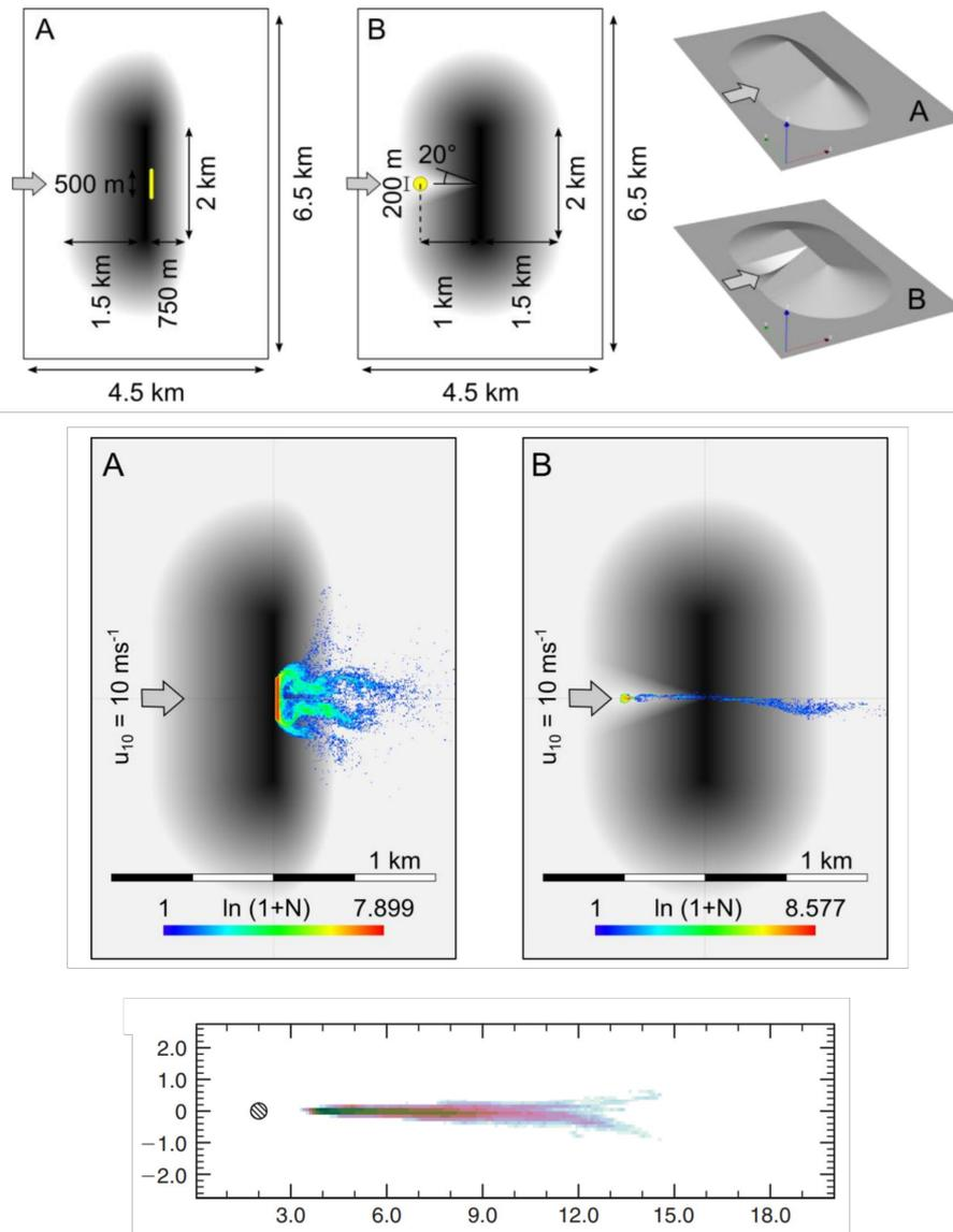
**FIGURE 21:** TOP ROW: TERRAIN AND FIRE CONFIGURATIONS CONSIDERED IN THE STUDY OF EMBER TRANSPORT IN THE PRESENCE OF COMPLEX TERRAIN FEATURES. THE TWO SCENARIOS ARE LABELLED AS ‘SCENARIO A’ AND ‘SCENARIO B’. MIDDLE ROW: DENSITY MAP OF FIREBRANDS FOR SCENARIO A AND SCENARIO B. BOTTOM ROW: EMBER DISTRIBUTION OBTAINED BY THURSTON ET AL. (2017) FOR THE CORRESPONDING WIND SPEED. FIGURES HAVE BEEN ADAPTED FROM HILTON ET AL. (2019A).
