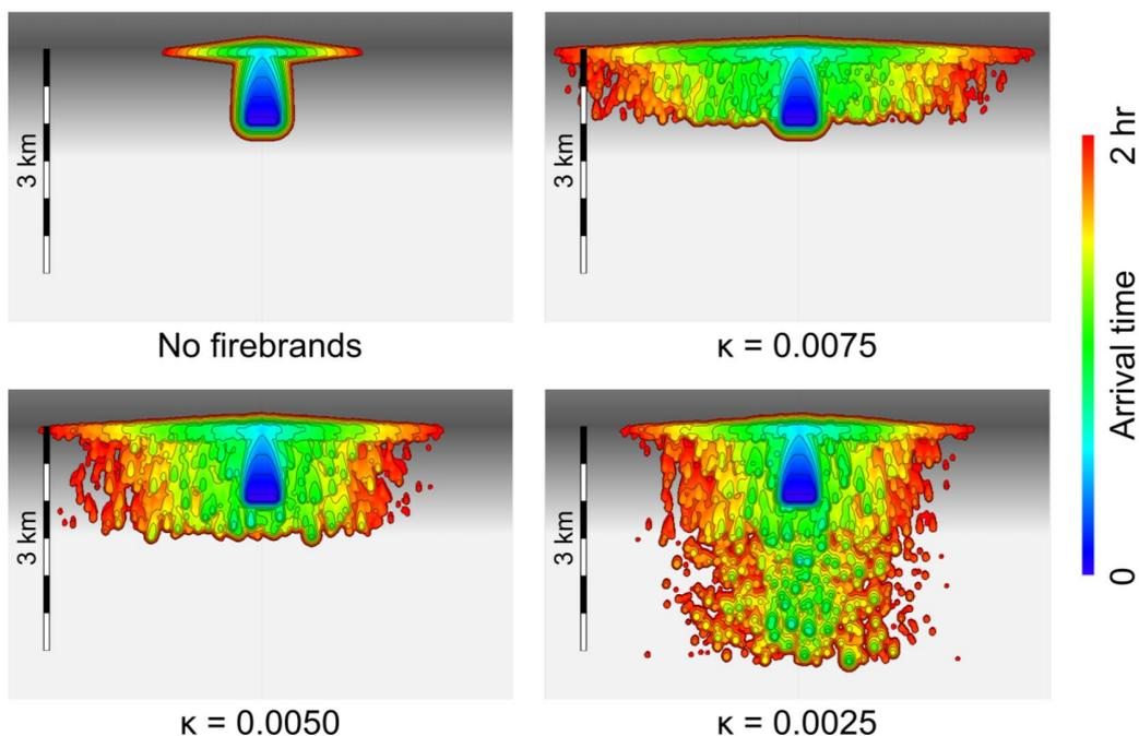
FIGURE 22: MODELLING VORTICITY-DRIVEN LATERAL SPREAD WITH AND WITHOUT FIREBRANDS AND FOR DIFFERENT VALUES OF THE PLUME COOLING PARAMETER  $\kappa$ , WHICH CONTROLS THE STRENGTH/BUOYANCY OF THE PLUME. FIGURE FROM HILTON ET AL. (2019B).
