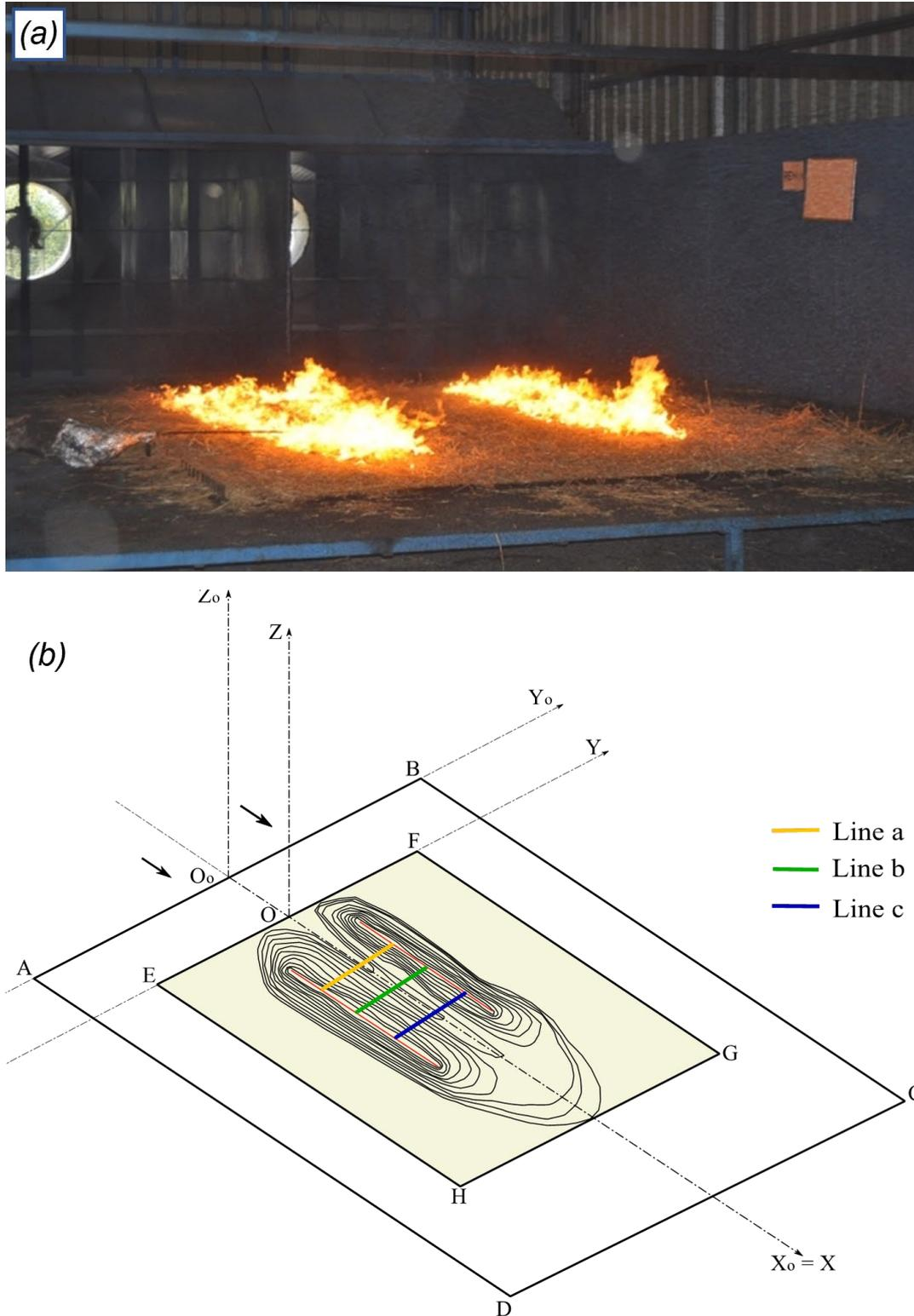
**FIGURE 18:** (A)VIEW OF THE COMBUSTION TUNNEL OF THE FOREST FIRE LABORATORY OF THE UNIVERSITY OF COIMBRA. (B) THE MEASUREMENT DIRECTIONS USED TO MEASURE THE RATE OF SPREAD OF THE APPROACHING FIRE LINES (LINES A, B AND C). THE ISOCHRONES CORRESPOND TO THE EXPERIMENT WITH THE FIRE LINES INITIALLY SEPARATED BY 1m AND WITH A WIND SPEED OF  $3 \text{ ms}^{-1}$ . THE FIGURES HAVE BEEN ADAPTED FROM RIBIERO ET AL. (2021).
