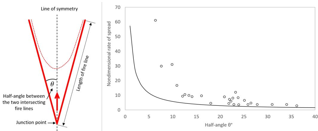
**FIGURE 2:** LEFT: SCHEMATIC REPRESENTATION OF THE JUNCTION FIRE CONFIGURATION SHOWING THE HALF-ANGLE  $\theta$ . RIGHT: EXPERIMENTAL CONFIRMATION OF DYNAMIC ENHANCEMENT OF THE RATE OF SPREAD. THE POINTS ARE THE OBSERVATIONS OF VIEGAS ET AL. (2012), WHILE THE SOLID LINE REPRESENTS THE ENHANCEMENT OF THE RATE OF SPREAD OF THE JUNCTION POINT EXPECTED DUE TO THE EFFECTS OF GEOMETRY ALONE.
