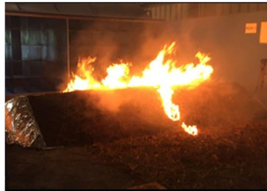
**FIGURE 19:** SCHEMATIC REPRESENTATION OF THE EXPERIMENTAL SETUP FOR THE EXPERIMENTS IN THE PRESENCE OF A MODEL HILL (TOP), THE ACTUAL EXPERIMENTAL SETUP IN THE WIND TUNNEL AT THE CENTRE FOR THE STUDY OF FOREST FIRES LABORATORY AT LOUSÁ, PORTUGAL, PRIOR TO IGNITION (BOTTOM LEFT), AND A PHOTOGRAPH OF ONE OF THE EXPERIMENTS WITH THE MODEL HILL, SHOWING THE INVOLVEMENT OF THE SPOT FIRES (BOTTOM RIGHT). THE FIGURE HAS BEEN ADAPTED FROM STOREY ET AL. (2021).
