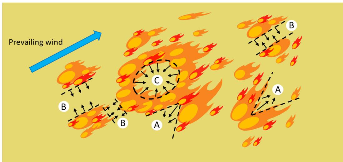
**FIGURE 1:** SCHEMATIC REPRESENTATION OF COALESCING SPOT-FIRES AND FORMS OF INTERACTION BETWEEN INDIVIDUAL SPOTS. EXAMPLES OF FIRE LINE INTERACTIONS INCLUDE (A) JUNCTION FIRES; (B) PARALLEL FIRE LINE MERGING; (C) PERIMETER COLLAPSE (RING FIRE). ALL OF THESE CONFIGURATIONS INVOLVE PYROCONVECTIVE INTERACTIONS THAT RESULT IN UNSTEADY FIRE SPREAD.
