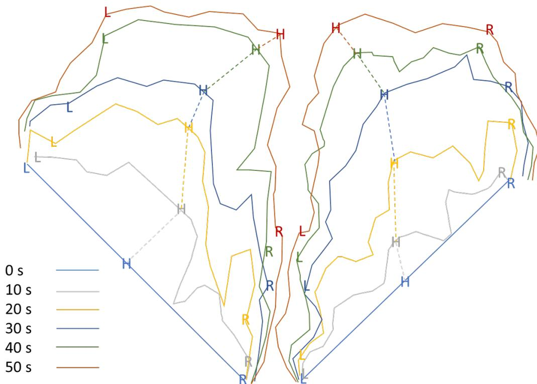
**FIGURE 13:** SCHEMATIC MAP OF FIRE ISOCHRONES BASED ON THE IMAGES PRESENTED IN FIGURE 1. LEFT FLANK (L), HEAD FIRE (H) AND RIGHT FLANK (R) POSITIONS ARE MARKED. DASHED LINES INDICATE TRAJECTORY OF EACH FIRE'S HEAD PATH BY ISOCHRONE.
