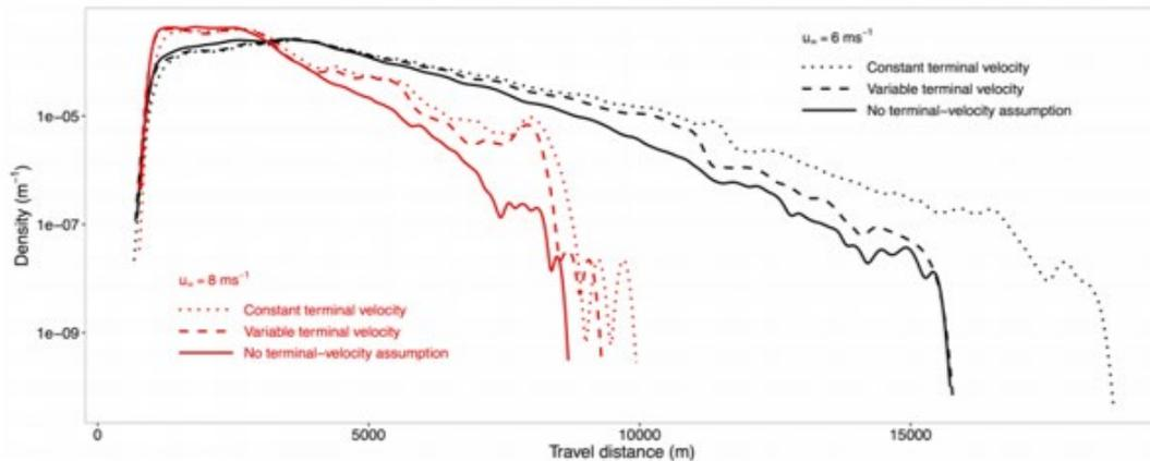
**FIGURE 20:** EFFECT OF THE TERMINAL VELOCITY ASSUMPTIONS ON EMBER DISTRIBUTIONS DERIVED FROM A COUPLED FIRE-ATMOSPHERE MODEL FOR TWO DIFFERENT AMBIENT WIND SPEEDS:  $6 \text{ ms}^{-1}$  (BLACK) AND  $8 \text{ ms}^{-1}$  (RED). DOTTED LINES REPRESENT THE DISTRIBUTION ASSUMING A CONSTANT TERMINAL VELOCITY, DASHED LINES REPRESENT VARIABLE TERMINAL VELOCITY AND SOLID LINES REPRESENT NO TERMINAL VELOCITY ASSUMPTION. FIGURE TAKEN FROM THOMAS ET AL. (2020).
