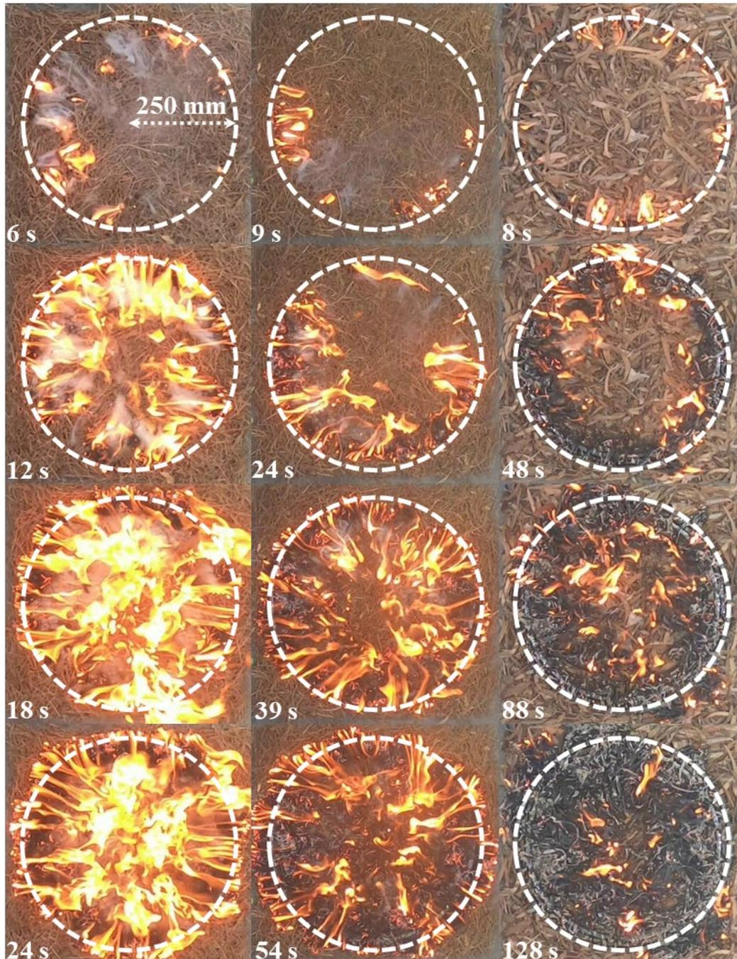
**FIGURE 14:** PLANAR IMAGERY AT VARIOUS TIMES SINCE IGNITION OF EXAMPLE ANNULAR FIRE EXPERIMENTS USING 500 MM DIAMETER IGNITION RING IN THREE FUEL CONDITIONS. (LEFT COLUMN) UNCOMPACTED PINE NEEDLES (LOW BULK DENSITY). (CENTRE COLUMN) COMPACTED PINE NEEDLES (INTERMEDIATE BULK DENSITY). (RIGHT COLUMN) UNCOMPACTED EUCALYPT LITTER (HIGH BULK DENSITY).
