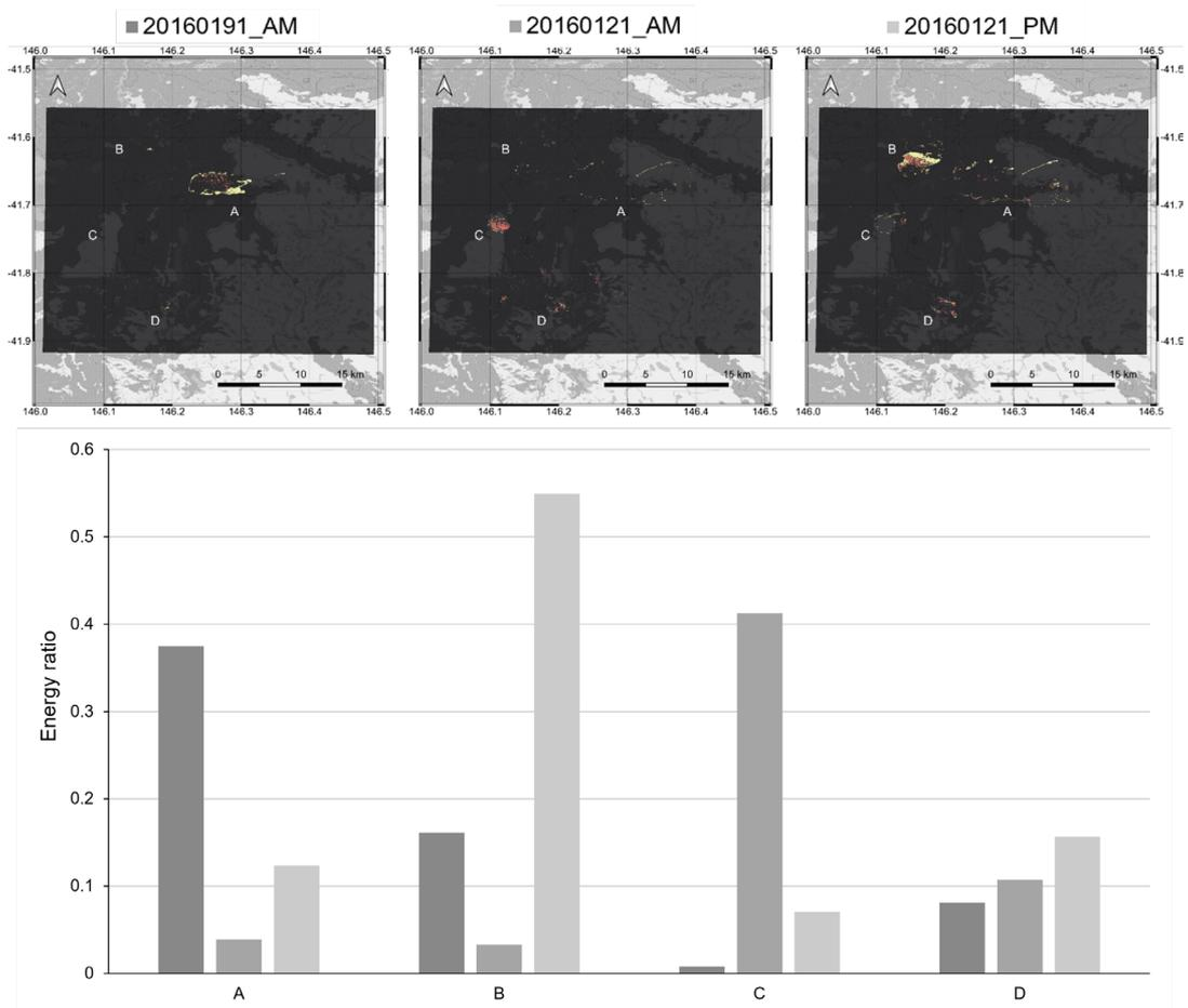
FIGURE 25: ENERGY RATIO INDEX VALUES FOR FOUR MOLE CREEK FIRES, LABELLED A, B, C AND D IN THE LINESCANS FOR THREE DIFFERENT TIMES: 19 JANUARY 2016 AM, 21 JANUARY 2016 AM, 21 JANUARY 2016 PM.
