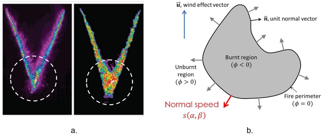
**FIGURE 3:** (A) INFRARED IMAGERY SHOWING THE ENHANCED RATE OF SPREAD OF THE JUNCTION POINT, WHICH IS ALSO THE POINT OF HIGHEST CURVATURE. FIGURE ADAPTED FROM VIEGAS ET AL. (2012). (B) SCHEMATIC REPRESENTATION OF A FIRE INTERFACE WITH LEVEL SET  $\phi$ , AND NORMAL SPEED  $s(\alpha, \beta)$ .
