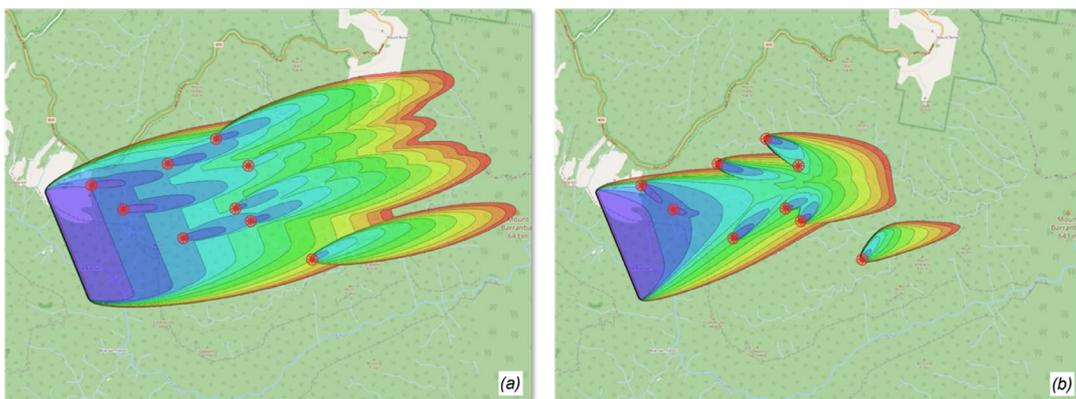
**FIGURE 11:** SPARK SIMULATION OF FIRE PROPAGATION RESULTING FROM A LINE IGNITION AND MULTIPLE SPOT IGNITIONS. (A) EVOLUTION OF THE FIRE IN THE ABSENCE OF PYROCONVECTIVE INTERACTIONS. (B) EVOLUTION OF THE FRONT INCORPORATING PYROCONVECTIVE INTERACTIONS. NOTE THE PRESENCE OF MULTIPLE JUNCTION FIRES IN THE SIMULATIONS.
