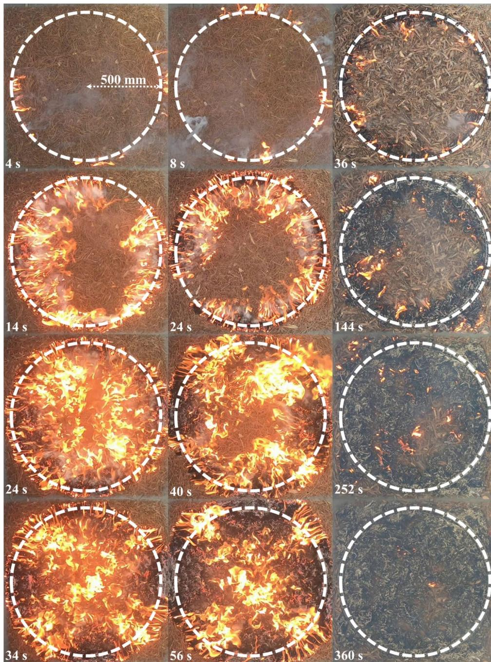
**FIGURE 15:** PLANAR IMAGERY AT VARIOUS TIMES SINCE IGNITION OF EXAMPLE ANNULAR FIRE EXPERIMENTS USING 1000 MM DIAMETER IGNITION RING IN THREE FUEL CONDITIONS. (LEFT COLUMN) UNCOMPACTED PINE NEEDLES (LOW BULK DENSITY). (CENTRE COLUMN) COMPACTED PINE NEEDLES (INTERMEDIATE BULK DENSITY). (RIGHT COLUMN) UNCOMPACTED EUCALYPT LITTER (HIGH BULK DENSITY).
