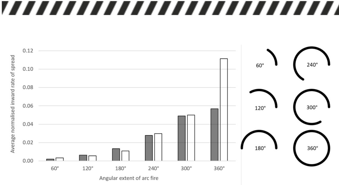
**FIGURE 5:** INWARD RATE OF SPREAD OF ARC FIRES SIMULATED USING A COUPLED FIRE-ATMOSPHERE MODEL. THE GREY SHADED BARS REPRESENT ARC FIRES WITH AN INITIAL RADIUS OF CURVATURE OF 1000 m, WHILE THE WHITE BARS REPRESENT ARC FIRES WITH AN INITIAL RADIUS OF CURVATURE OF 500 m (THOMAS 2019). THE VARIOUS ARC FIRES CONSIDERED ARE SHOWN TO THE RIGHT.
