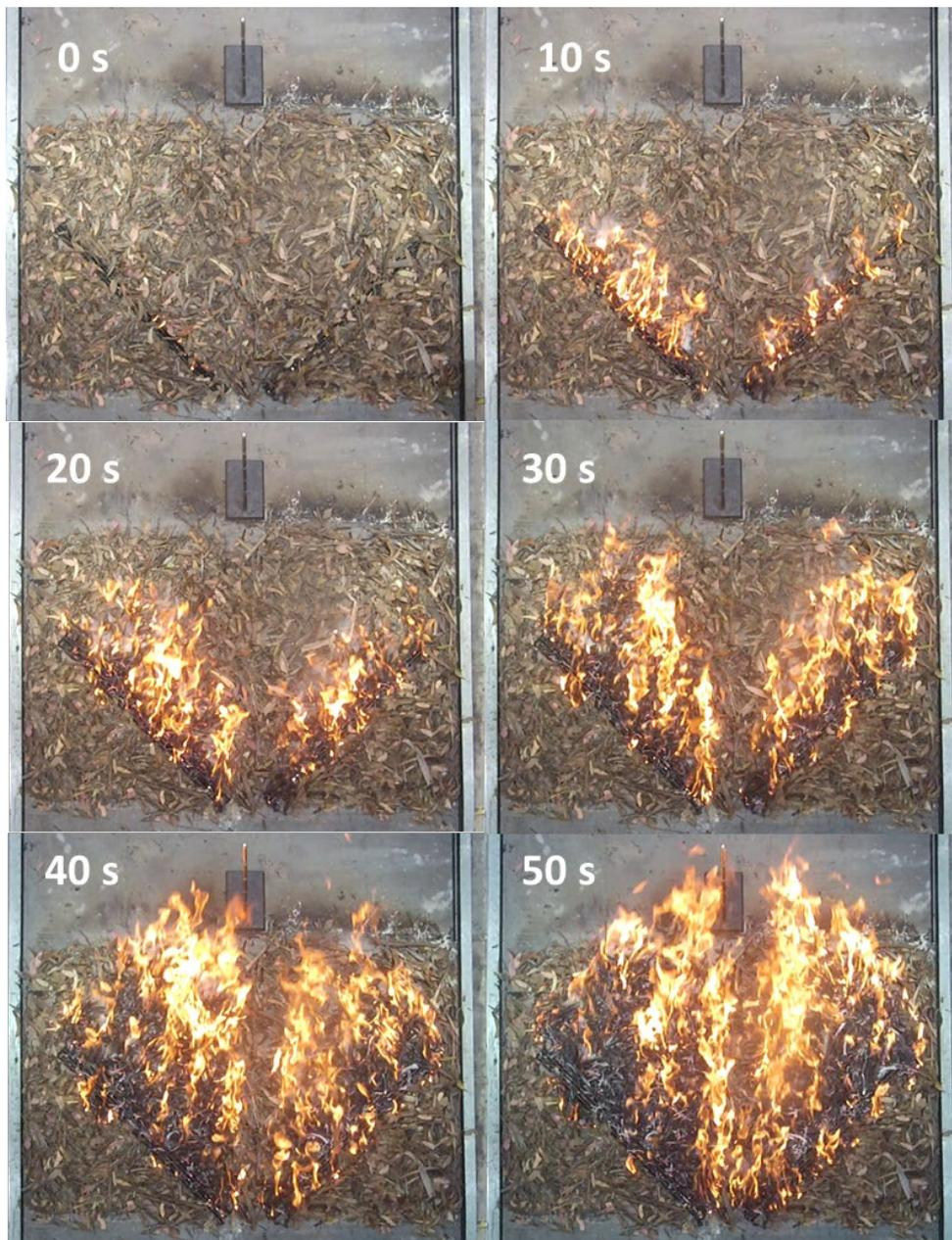
**FIGURE 12:** EXAMPLE OF A SEPARATED 'V' FIRE AT VARIOUS TIMES SINCE IGNITION IN WHICH TWO 800 MM IGNITION LINES AT AN INTERSECTION ANGLE NORMAL TO THE FLOW OF 1 M/S AIR (BOTTOM OF FRAME TO TOP) IS 45°. AS CAN BE SEEN, THE FIRE FROM EACH IGNITION LINE DEVELOPS INDIVIDUALLY, ONLY MERGING AFTER 50 SECONDS. HOWEVER, THE HYPOTHESIS OF THE EXPERIMENT IS THAT THE BEHAVIOUR OF EACH FIRE IS DIFFERENT FROM THAT OF A SINGLE FIRE.
