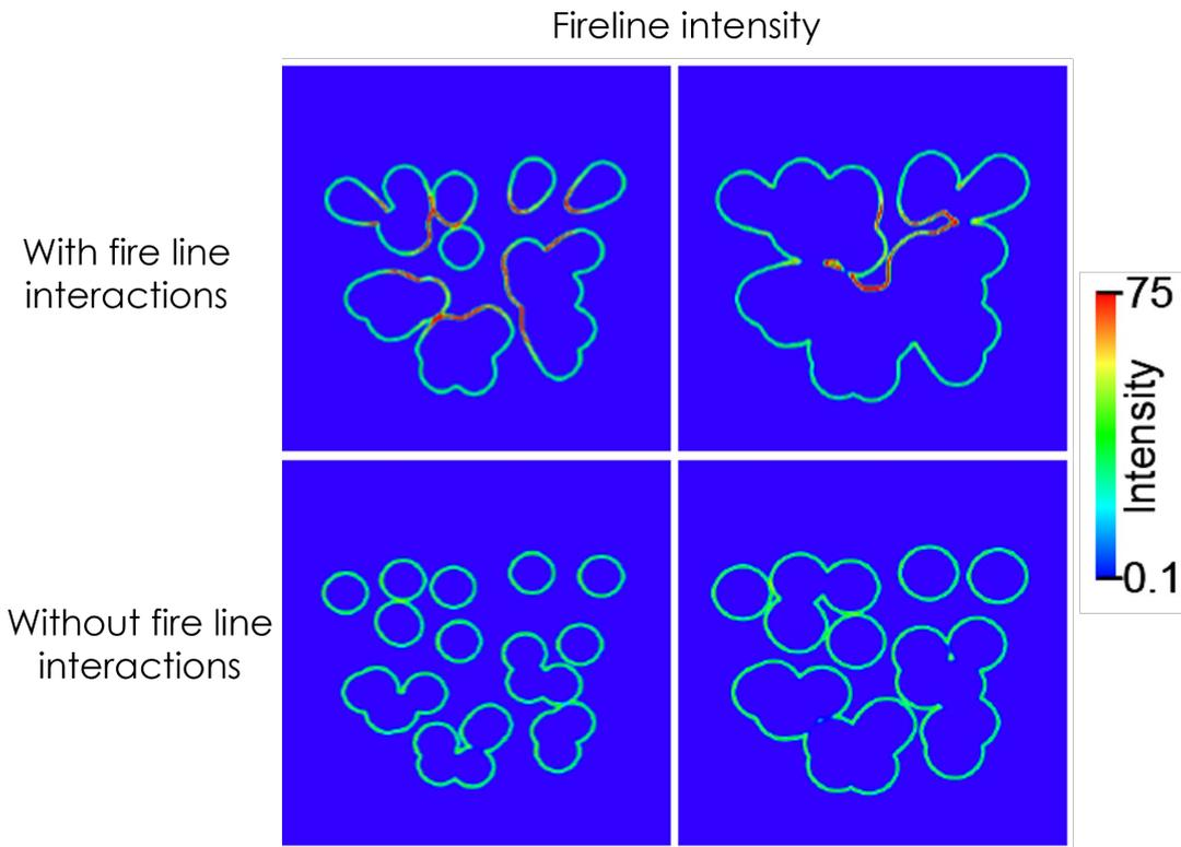
**FIGURE 9:** COALESCENCE OF 25 SPOT FIRES WITH (TOP ROW) AND WITHOUT (BOTTOM ROW) PYROCONVECTIVE INTERACTION, THE LEFT COLUMN SHOWS THE DEVELOPMENT OF THE FIRES 15 SECONDS AFTER IGNITION AND THE RIGHT COLUMN SHOW THE FIRES 20 SECONDS AFTER IGNITION. RED COLOURS INDICATE LOCAL ENHANCEMENTS IN (NON-DIMENSIONALISED) FIRE INTENSITY DUE TO PYROCONVECTIVE EFFECTS. FIGURE ADAPTED FROM HILTON ET AL. (2017)
