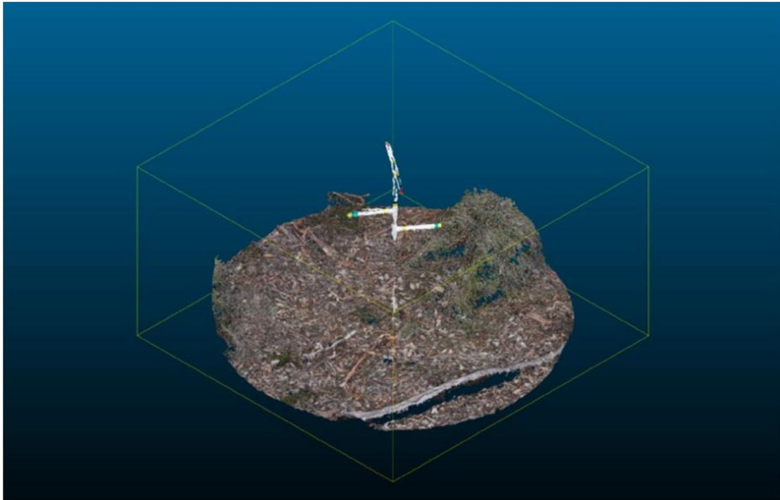
FIGURE 8. VOXELLISED DENSE POINT CLOUD IN POINT CLOUD PROCESSING SOFTWARE CLOUDCOMPARE.
