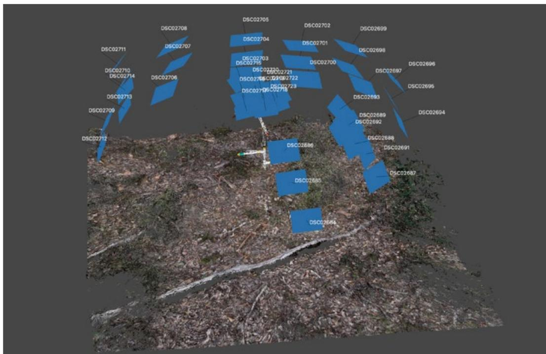
FIGURE 7. VIEW OF DENSE POINT CLOUD, WITH ASSOCIATED CAMERA GEOMETRY WITHIN METASHAPE PRO.
