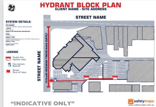
Block Plans that can be printed on any medium of your choice, PVC, Brushed Alloy or Anodised. A3 displaying all necessary information about the buildings hydrant system.
