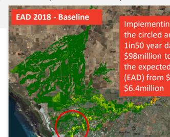
Implementing a floodway in the circled area reduces the 1in50 year damage from \$98million to \$73million and the expected annual damage (EAD) from \$7.3million to \$6.4million
